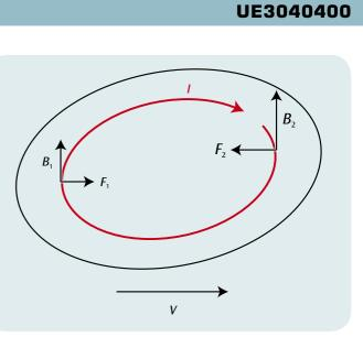
Eddy current *I* in a metal disc moving at speed *v* through a uniform magnetic field  $B_1$ ,  $B_2$  with Lorentz forces  $F_1$  and  $F_2$  acting on both limbs of the eddy. The force acting against the motion is greater than that operating in the same direction.
