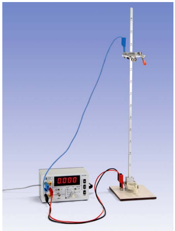
Fig. 1: Experiment set-up for measuring the fall time of a steel ball as a function of the distance h between the trigger mechanism and a target plate.
