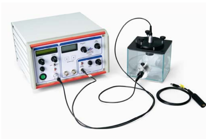
Fig. 3: Experiment set-up for the diffraction of light at a phase grating produced in a liquid by ultrasonic waves
