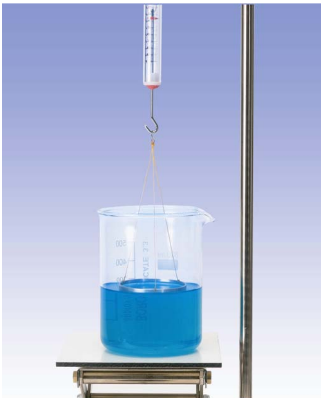
Fig. 3: Experiment set-up for surface tension measurements
