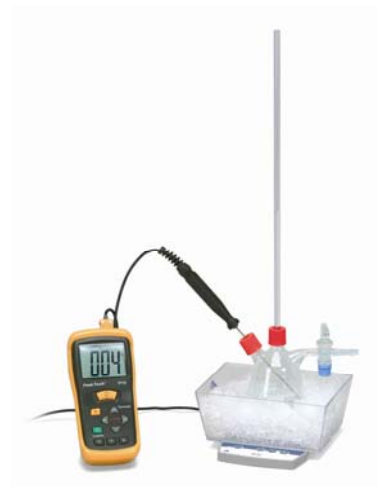
Fig. 2: Experiment set-up for determining the temperature of the maximum density of water
