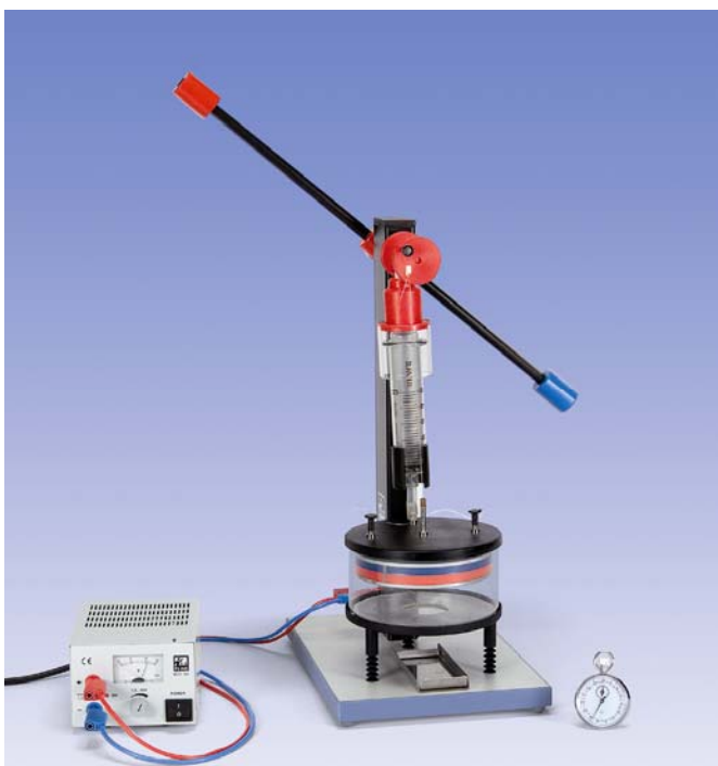
Fig. 5: Set-up for the operation of a Stirling engine as a heat engine by means of electric heating
