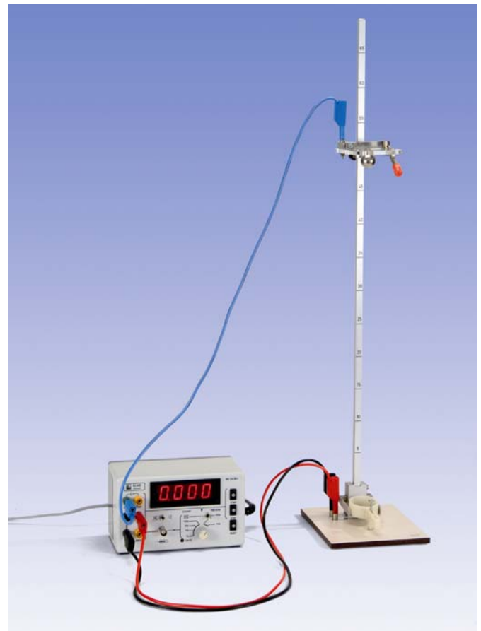
Fig. 1: Experiment set-up for measuring the fall time of a steel ball as a function of the distance h between the trigger mechanism and a target plate.
