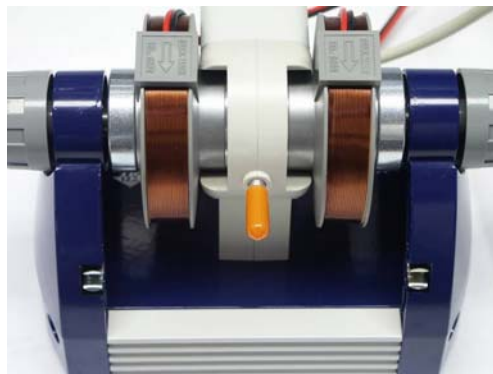
Fig. 4 Basic unit with DPPH sample inserted
