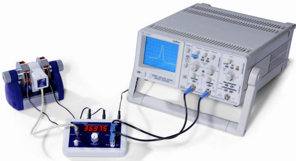
Fig. 5 ESR experiment set-up using an oscilloscope
