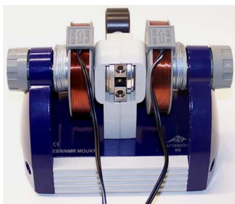
Fig. 6 Basic unit completed with permanent magnets and coils
