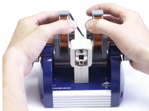
Fig. 4 Pulling the two permanent magnets apart
