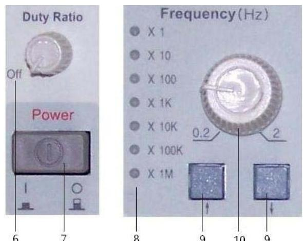
6 Adjustment knob for duty ratio. In "OFF"-position the signal is symmetrical
