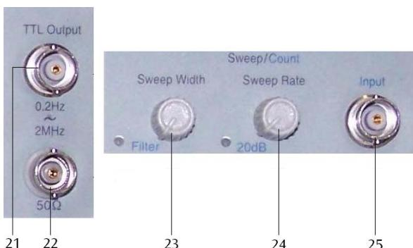
21 Output socket for standard TTL signal, impedance 600 Ω
