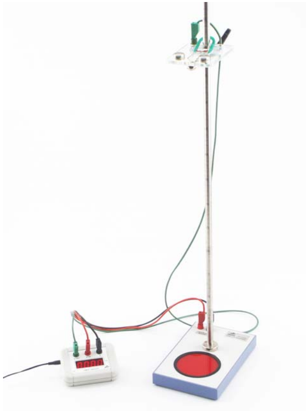
Fig 2 Millisecond counter and free fall apparatus
