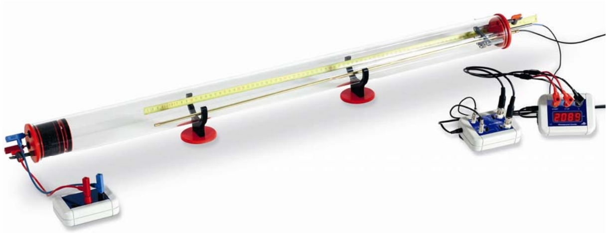
Fig. 2: Experiment set-up with Kundt's tube
