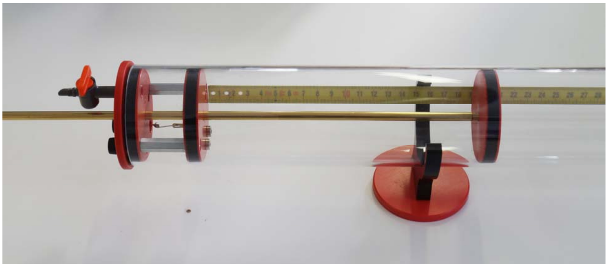
Fig. 1 Microphone probe with sensor disc screwed on
