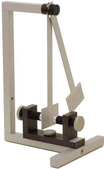
Fig. 5: Experiment set up for "induced eddy currents"
