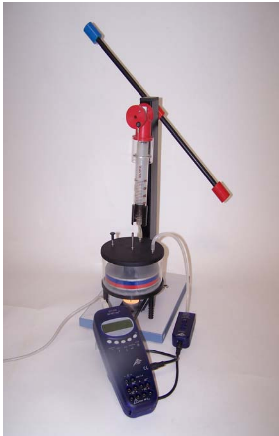
Fig. 1 Experiment set-up for recording operating pressures in the Wilke-type Stirling engine while in motion
