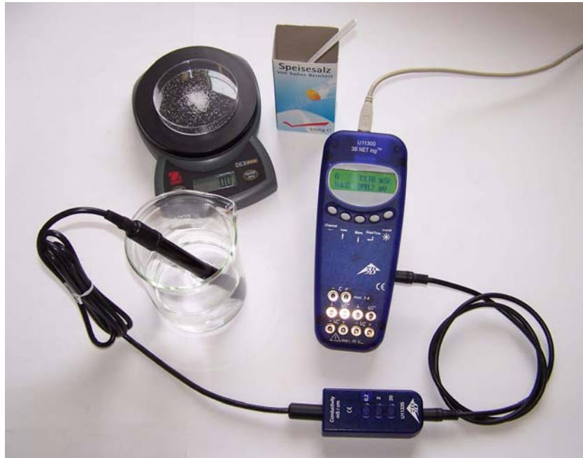
Fig. 1 Set-up for increase in conductivity of distilled water due to addition of common salt
