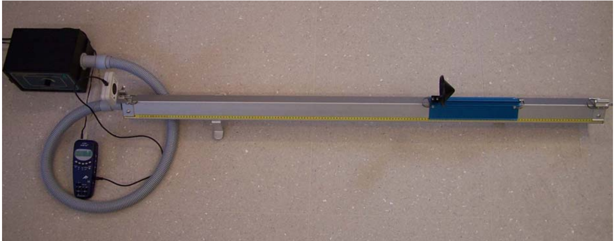
Fig. 1: Experiment set-up for measuring speed on an air track
