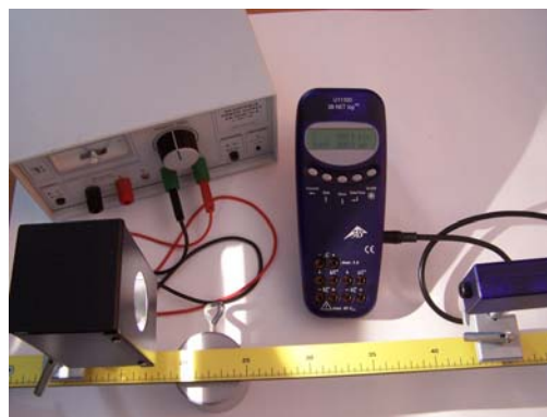
Fig. 1 Investigation of the inverse square law for a point light source
