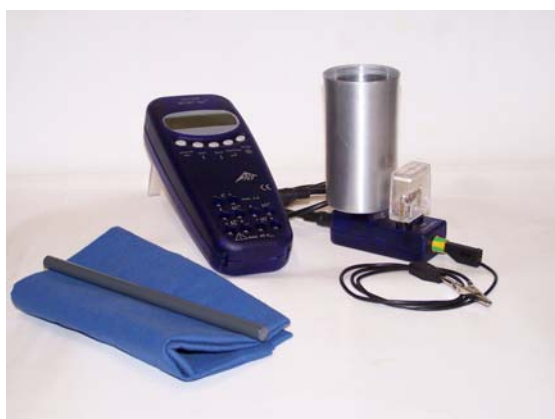
Fig. 1 Experiment set-up for measuring charges in electrostatics
