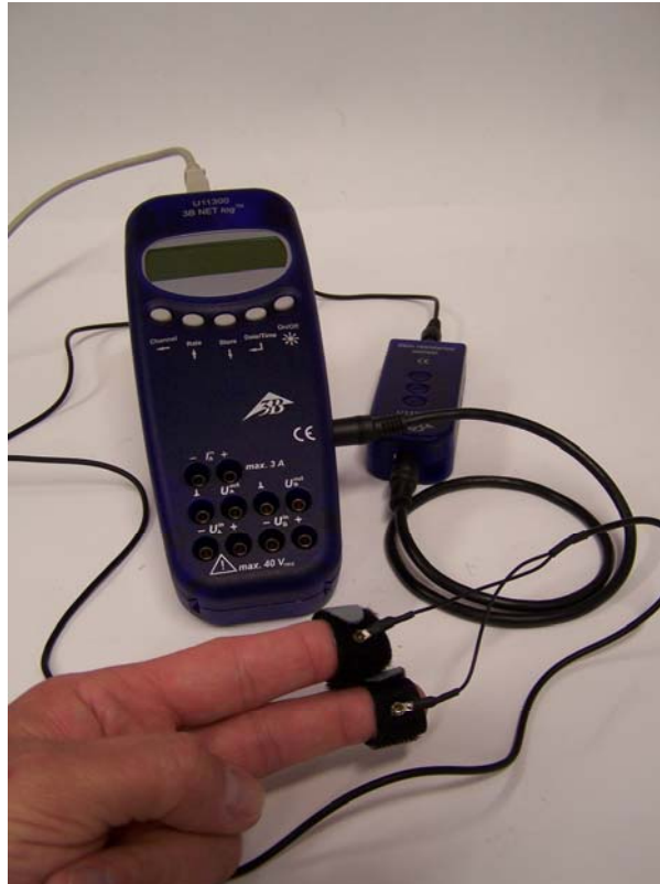
Fig. 1 Measuring skin resistance of a person
