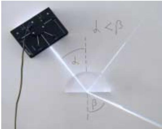
**Exp.11: Semi-circular body - Light incident at right angle to tangent**
