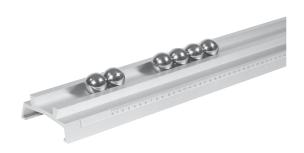
Steel balls suitable for experiments on elastic and inelastic collisions on a slide rail.
