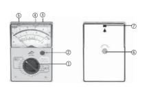
Handheld meter used to measure current, voltage and resistance as well as gain levels or attenuation e.g. in chains of quadripoles.
