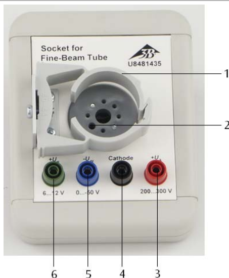
Fig. 1 Socket: 1 Clip, 2 Opening for guide pin, 3 connection for anode, 4 connection for cathode, 5 connection for Wehnelt cylinder, 6 connection for heater
