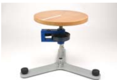
Fig.4 Determination of the moment of inertia of a wooden disc
