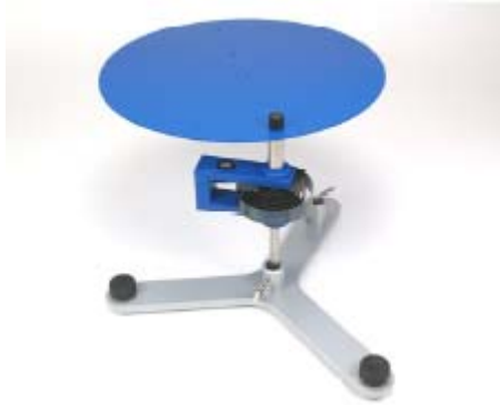
Fig. 7 Verification of Steiner's theorem
