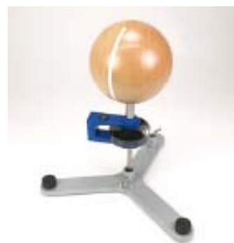
Fig. 6 Determination of the moment of inertia of a sphere
