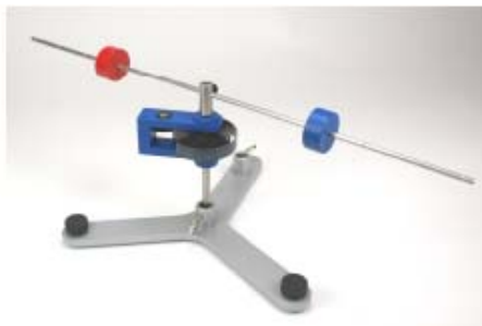
Fig. 3 Dependency of the moment of inertia J on the distance r
