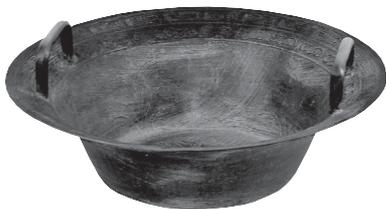
The resonance basin is used to demonstrate stationary waves in a bronze bowl filled with water.
