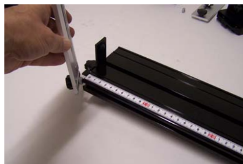
Fig. 14 Inserting the holder for light barrier into the groove at the side of the trolley track
