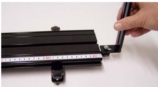
Fig. 8 Inserting the holder for pulley into the middle groove at the bottom side of the trolley track
