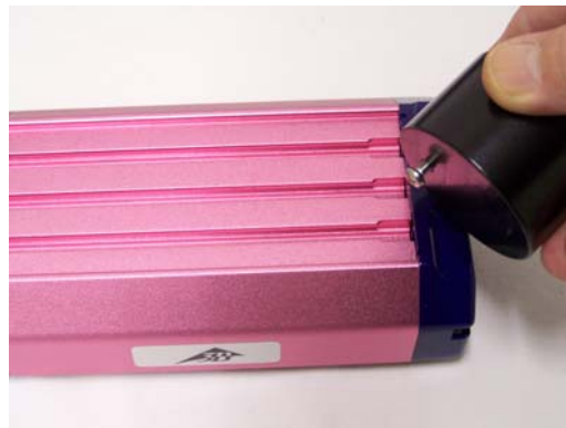
Fig. 21 Inserting the additional weight into the groove on the upper side of the trolley
