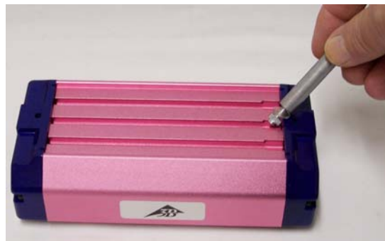
Fig. 23 Inserting the contact-breaker into the groove on the upper side of the trolley
