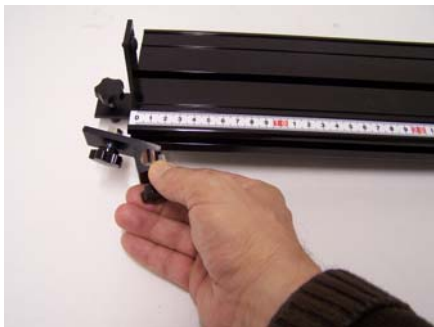
Fig. 18 Inserting the rod clamp into the groove at the side of the trolley track
