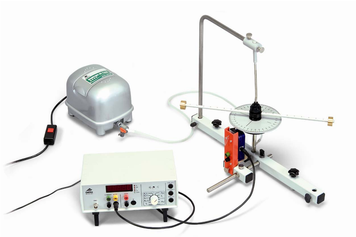
Fig. 2 Experiment set-up for determining moment of inertia of transverse beam with additional masses, using a laser reflection sensor (U8533380) and a digital counter (U8533341).
