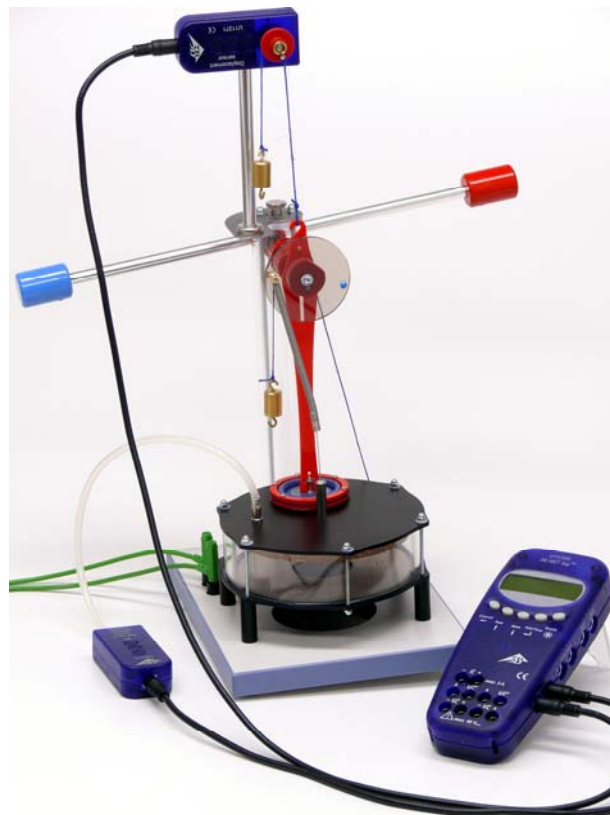
Fig. 8 Set-up for recording a pressure-volume diagram
