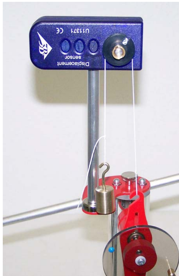
Fig. 5 Attaching the thread to the hook on the connector rod
