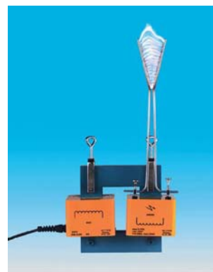
Spark discharge along horn-shaped electrodes
