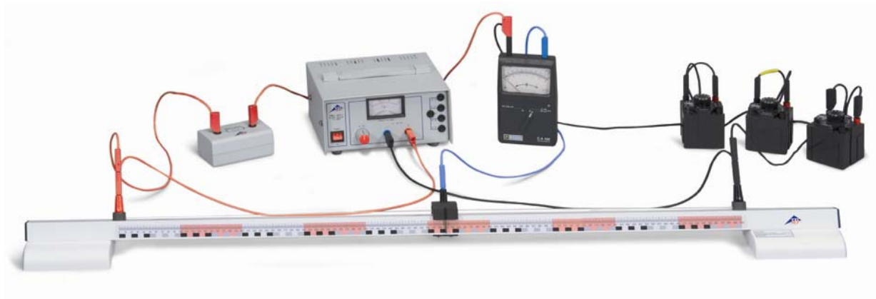
Fig. 2 Determining resistance in a Wheatstone bridge circuit
