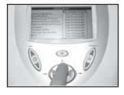
4. Press the DUTY CYCLE (up arrow) or FREQUENCY (down arrow) buttons to highlight Unit Default Protocol.
