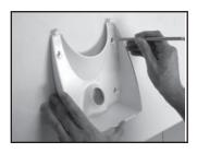
2. Using the bracket as a guide, mark the 4 wall holes with a pencil or pen.
