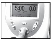
3. Press the Duty Cycle (up arrow) button to select 10%, 20%, 50% or Continuous duty cycle. When the button is pressed, an audible tone will be heard as the duty cycle toggles through the options on the LCD.
