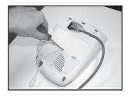
Locate the battery access door at the bottom of the unit and loosen the screw with a regular screwdriver.
