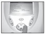
3. Press the DUTY CYCLE (up arrow) and FREQUENCY (down arrow) buttons to highlight Save Protocol, and press the DISPLAY (enter) button to accept the highlighted selection.
