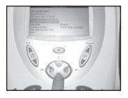
2. Press the DUTY CYCLE (up arrow) or FREQUENCY (down arrow) buttons to highlight the Restore Factory Protocols option.
