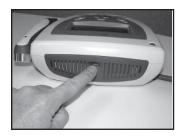
To brighten or dim the LCD, turn the contrast control dial until the display contrast is optimal.
