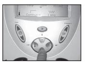
2. Press the Frequency button to select 1 or 3.3 MHz. When the button is pressed, the frequency will toggle from 1 to 3.3 MHz and back again as long as the button is being pressed.
