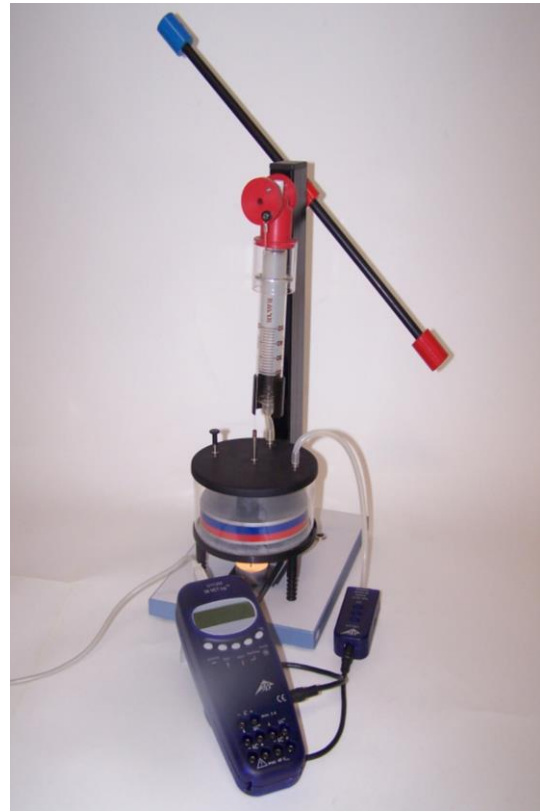
Fig. 1 Experiment set-up for recording operating pressures in the Stirling engine D while in motion
