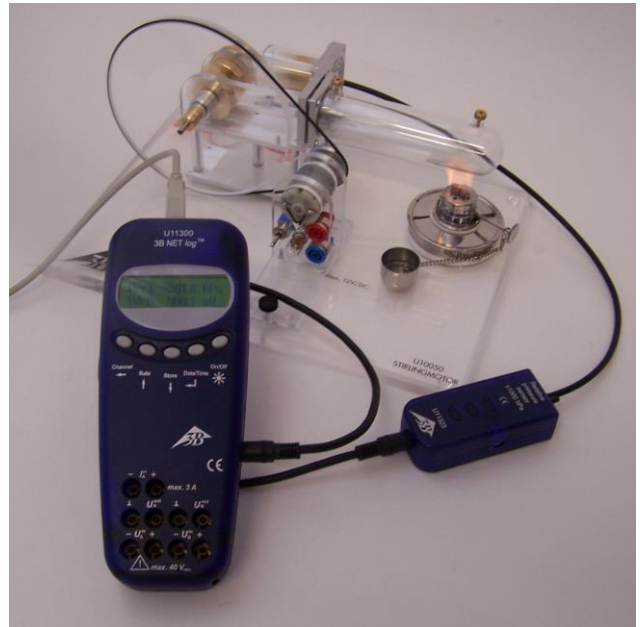
Fig. 1 Experiment set-up for recording operating pressures in Stirling engine 1002594 while in motion
