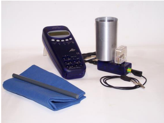
Fig. 1 Experiment set-up for measuring charges in electrostatics
