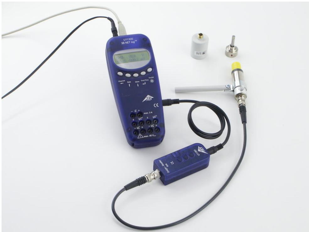
Fig. 1 Experiment set-up for recording decay events in the beam from a radioactive source
