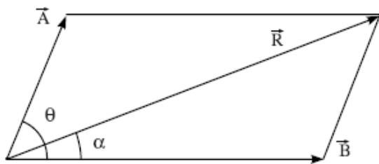
This theorem can be expressed mathematically as follows: When two forces  $\vec{A}$  and  $\vec{B}$  acting on a body with an angle  $\theta$  between them, the resultant  $\vec{R}$  is given by:
