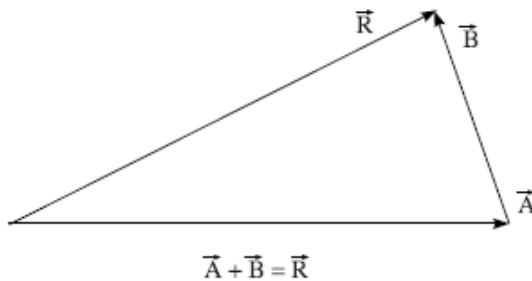
From this it can be determined that a body is in equilibrium if three forces are acting upon it, which can be represented by the three sides of a triangle. If more than two forces act on a body at once, the law of the polygon of forces is used. This represents several forces acting at the same point as following sides of a polygon where one side remains open. As for the triangle, following the side that closes the polygon in the opposite direction gives the resultant force.
