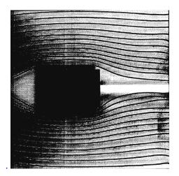
When air flows past a rectangular body, the flow lines narrow around the body itself. The velocity of flow also increases. Once the flow passes the body, the flow velocity reduces.
