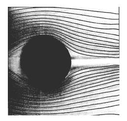
When air flows around a circular or spherical body, the flow lines narrow around the body itself. The velocity of flow also increases. Once the flow passes the body, the flow velocity reduces.
