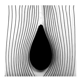
When the air flow moves around a teardropshaped body, the flow lines narrow around the body itself. The velocity of flow also increases. Once the flow passes the body, the flow velocity reduces. 5.3 Course of flow around a spherical body
