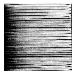
In the case of linear laminar flow, all flow lines are parallel. The direction and flow velocity are equal at all points of the air flow.
