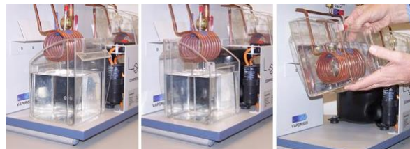
Fig. 3 Connection of the water reservoirs to the heat pump Left: reservoir with its lower edge facing the pump Centre: reservoir turned with its lower edge facing the front Right: reservoir suspended in holding plate
