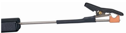
Fig. 2 Pt 100 thermocouple with measurement terminal
