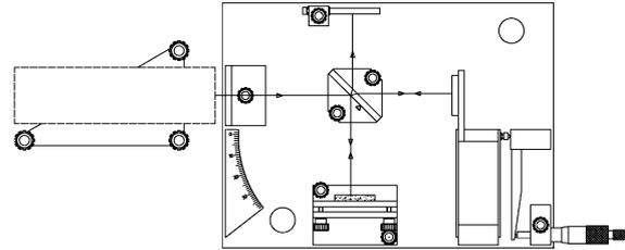
Fig. 2 Experiment setup for the Michelson Interferometer
