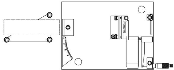
Fig. 6 Experiment setup for Fabry-Perot interferometer.
