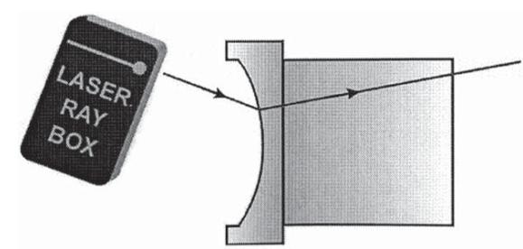
**E13b Light beam passing through convex air-glass boundary**
