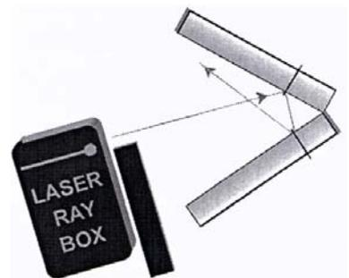
**E3a Reflection of light rays on concave mirror – rays are parallel to optical axis**
