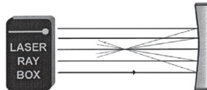
**E3b Reflection of light rays on concave mirror – rays are non-parallel to optical axis**
