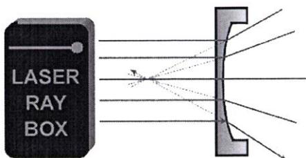
**E16b Light beam passing through concave glass-air boundary**
