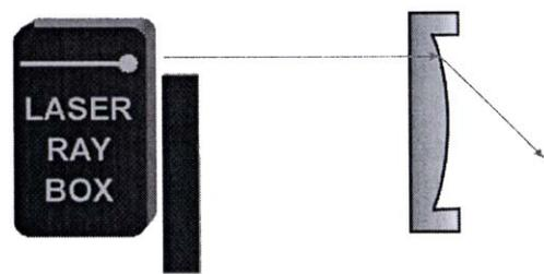
**E15b Light beam passing through convex glass-air boundary**
