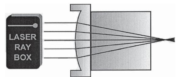
**E14b Light beam passing through concave air-glass boundary**
