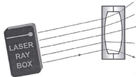
**E20a Light beam passing through air concave lens – the rays are parallel to the optical axis**
