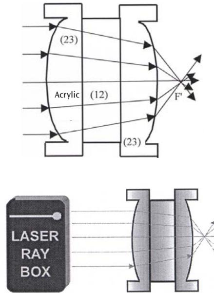
**E18a Light beam passing through glass concave lens – the rays are parallel to the optical axis**
