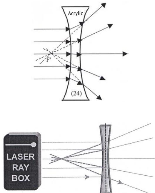
**E18b Light beam passing through glass concave lens – the rays are non-parallel to the optical axis**
