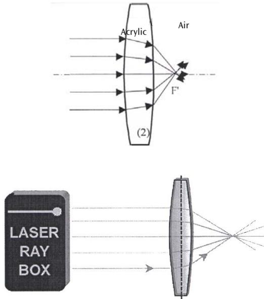
**E17b Light beam passing through glass convex lens – the rays are non-parallel to the optical axis**
