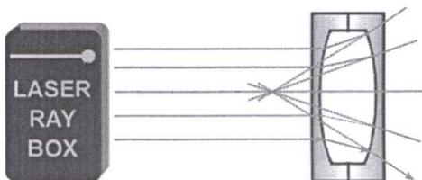
**E19b Light beam passing through air convex lens – the rays are non-parallel to the optical axis**
