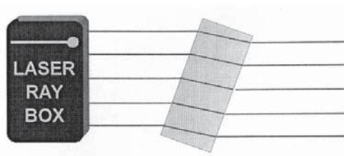
**E8 Light ray shift by air planparallel plate**
