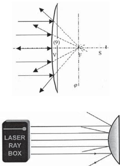
**E4b Reflection of light rays on convex mirror – rays are non-parallel to optical axis**
