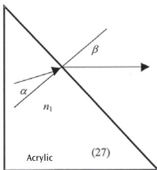
**E6d Total reflection – propagating of light in optical fibres**
