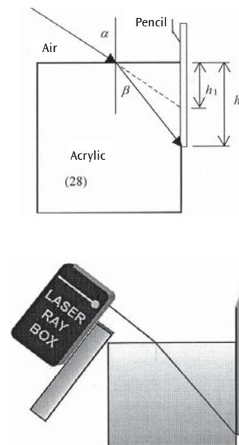
**E6a Refraction of light passing glass-air boundary**
