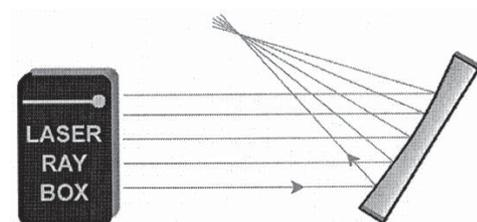
**E4a Reflection of light rays on convex mirror – rays are parallel to optical axis**
