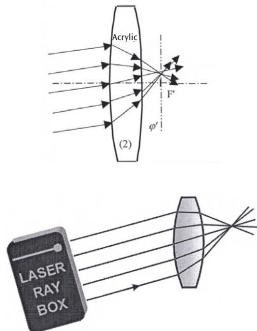
**E17c Light beam passing through thick glass convex lens**
