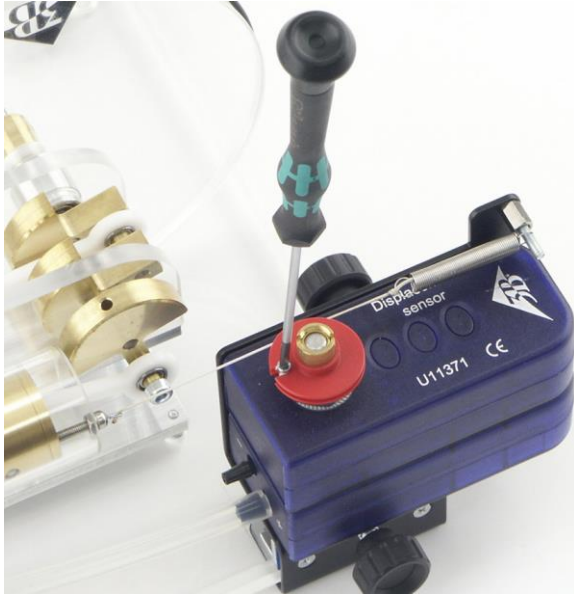
Fig. 8 Securing the string
