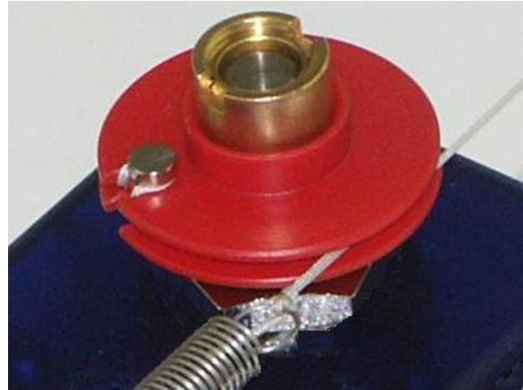
Fig. 5 How the string is threaded around the pulley
