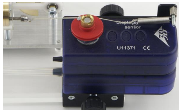
Fig. 7 Poorly aligned sensor holder whereby the string sags at full extension
