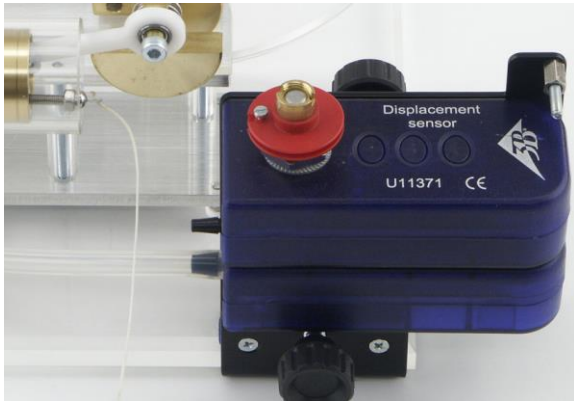
Fig. 3 Attachment of string to working piston and assembly of displacement sensor
