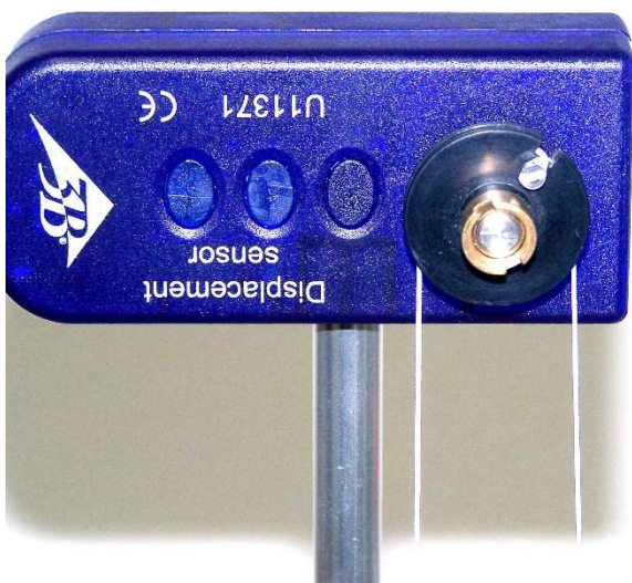
Fig. 3: How the thread is wound around the pulley
