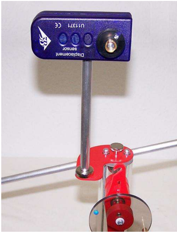
Fig. 2: Assembly of displacement sensor
