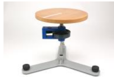
Fig. 4 Determination of the moment of inertia of a wooden disc
