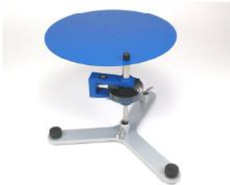
Fig. 7 Verification of Steiner's theorem
