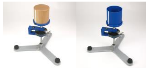
Fig. 5 Comparison of the moments of inertia of cylinders
