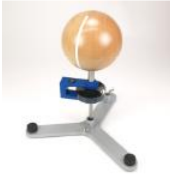
Fig. 6 Determination of the moment of inertia of a sphere
