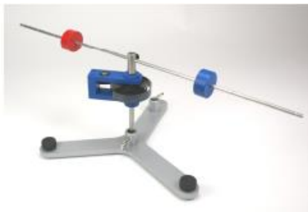
Fig. 3 Dependency of the moment of inertia J on the distance r
