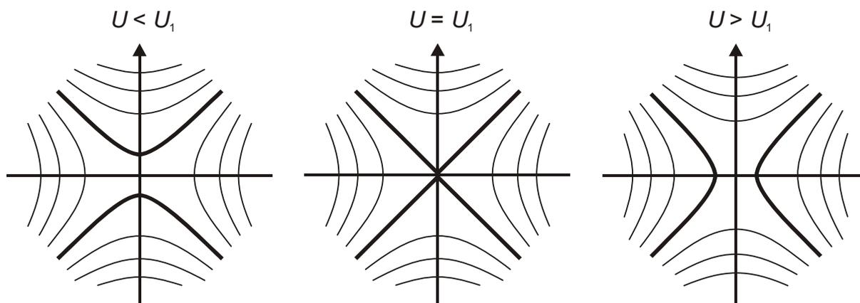
Fig. 3: Change in interference pattern due to Pockels effect. The hyperbolae highlighted bold are those of interference order +1.
