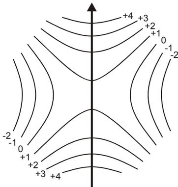
Fig. 2: Interference pattern with the optical axis of the crystal shown by the arrow. The indices of the dark interference lines indicate the path difference between the ordinary and extraordinary rays using the wavelength of the incident light as a unit.
