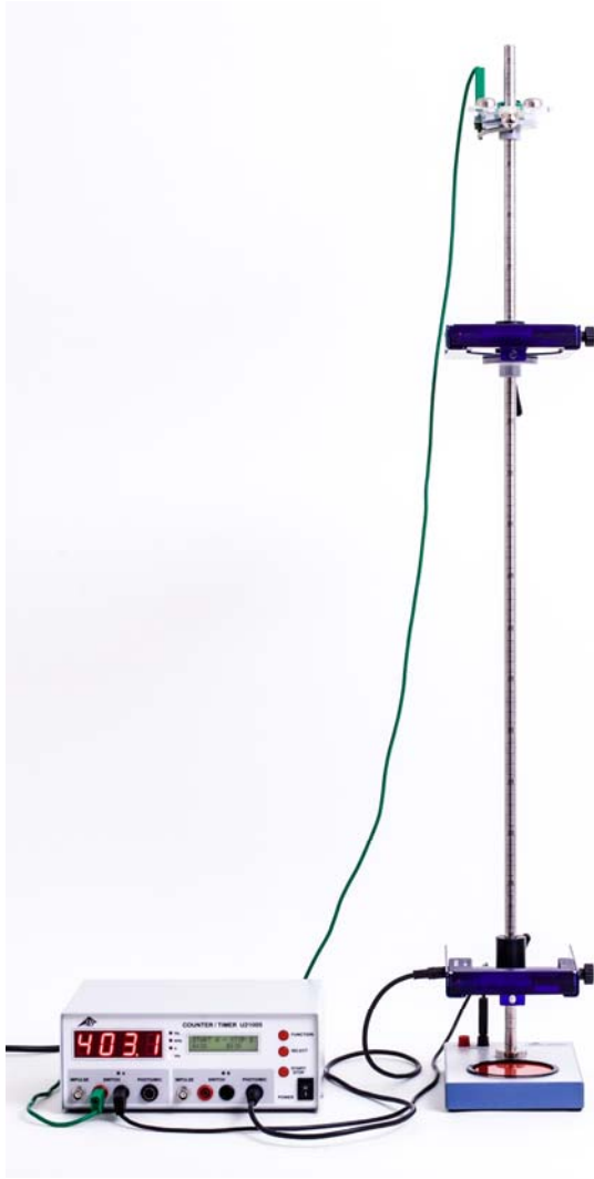
Fig. 2: Experiment set-up for measuring average velocity.
