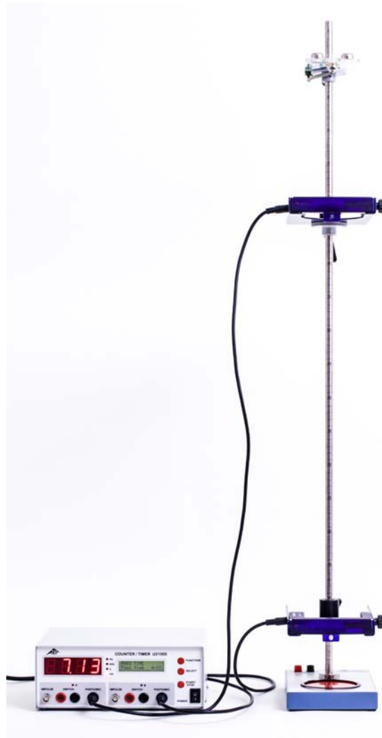
Fig. 1: Experiment set-up for measuring instantaneous velocity.
