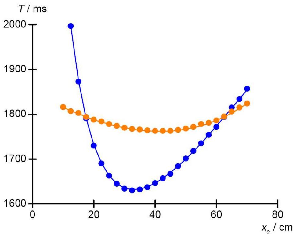
Fig. 6: Period of oscillation  $T$  as a function of the distance  $x_2$  of the moving pendulum bob from the suspension point (the bearing fulcrum). Red circles: Both pendulum bobs below fulcrum. Blue circles: Fixed pendulum bob above fulcrum, movable bob below
