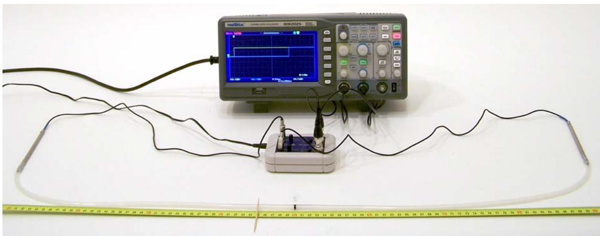
Fig. 3: Measurement of difference in time for sound to reach two microphones using an oscilloscope.
