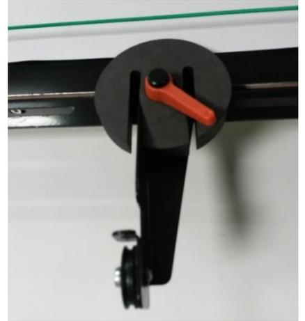
*Offset pulley fitted to one of the table brackets supplied
