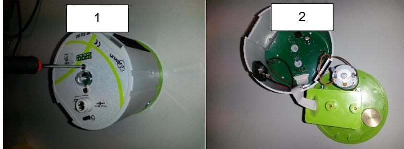
**Warning: the removal of the hood should be no sudden move to avoid breaking flouder**
