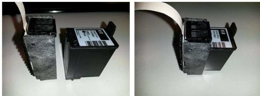
2. Pass the connector through the window of the L-bracket with Velcro, then velcro the cartridge holder in the L-bracket.
