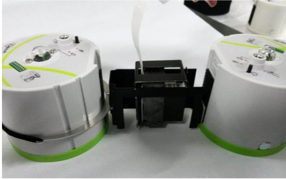
5. Connect this marking accessory over the top of the puck containing an ink cartridge (see picture below).
