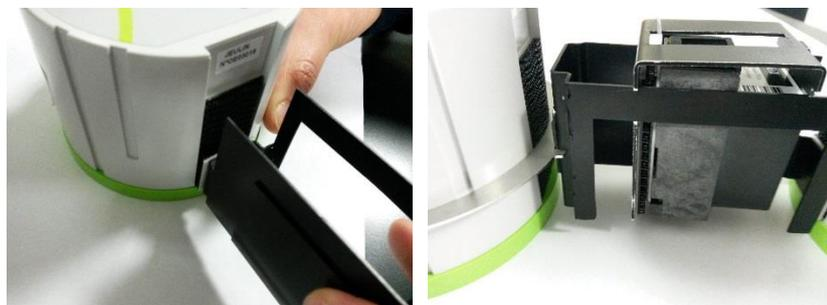
4. Slide the assembly with ink cartridge into the rectangle.
