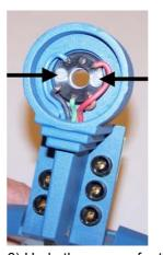
6) Undo the screws for the contact ring.
