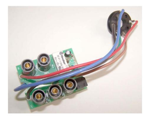
The quality of the electron beam in electron deflection tube S (1013889) is affected by the resistance between sockets C5 (cathode) and F4 (heating filament) on the tube. For optimum results, the resistance  $R_{\text{C5F4}}$  needs to be 390 k $\Omega$ . Tube holder S (1014525) is accordingly designed such that this resistance is present.
